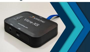
**Vitra-XS** is Ashling's Debug & Trace Probe for embedded development with support for multiple target architectures including RISC-V, Arm-Cortex, MIPS (P8700 & I8500) & Synopsys ARC-V & ARC powered systems.
