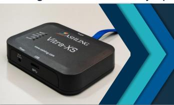
**Vitra-XS** is Ashling's Debug & Trace Probe for embedded development with support for multiple target architectures including Synopsys ARC-V & ARC powered systems.
